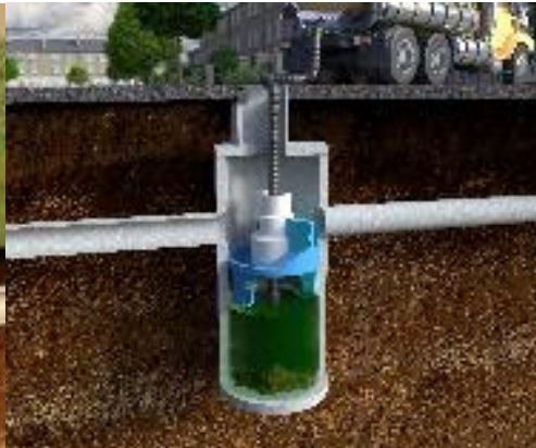
Oil Grit Separator
