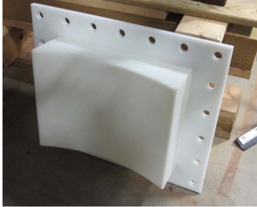
Figure 7 Sump Access Port sits Flush with Interior Manhole Wall
