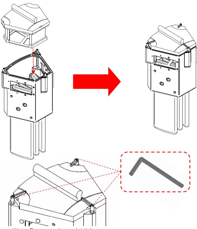
\*Note: Ensure each cam latch is centered over its corresponding indentation in the Filter Module Lid before fully tightening.
