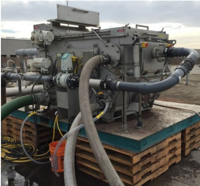
A Hydro MicroScreen™ MS-28 unit was tested against existing technology in a season-long trial
