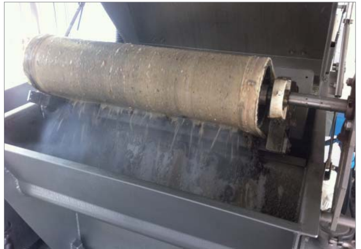
Hydro MicroScreen Rotating Belt Reduces BOD and Gets More TSS
