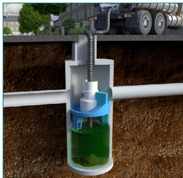
Fig 3. Maintenance is done with a vactor truck
