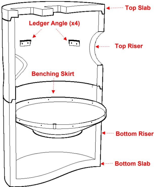
8ft. Downstream Defender consisting of bottom slab, bottom riser (with benching skirt) top riser (with ledger angle) and top slab.
