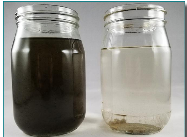
Before and after shots show the effectiveness of chemical flocculents in reducing turbidity
