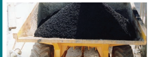
Clean, dewatered grit ready for disposal.
