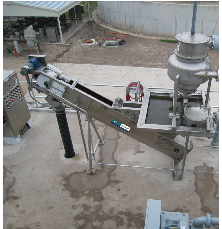
Installed TeaCup® / Grit Snail® system
