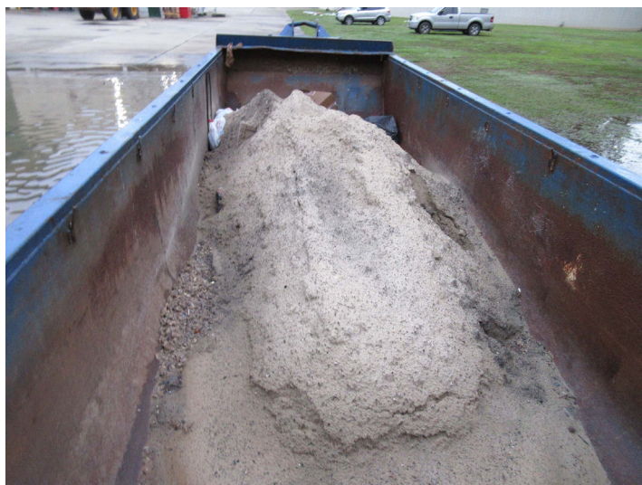
Grit Dumpster Load on May 26, 2020 After Only 0.2" (5 mm) of Rain
