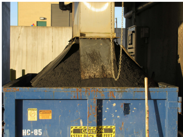
Grit Dumpster Load Midway Through Storm with 3" (7.6 cm) of rain
