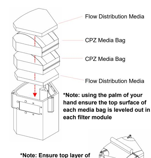
flow distribution media is leveled out below the conveyance channels and the Filter Module Lid forms a
