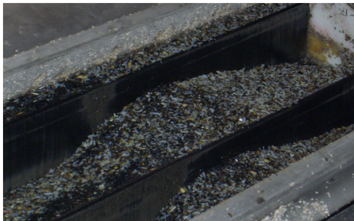
Grit Removed from Rock Creek's Sludge
