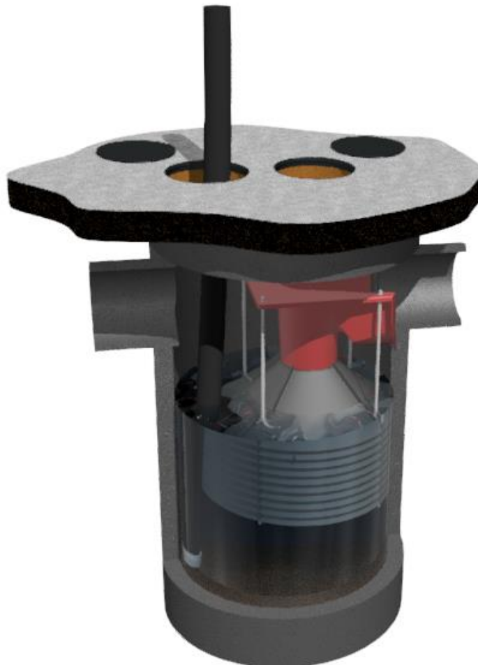
Fig.4 Floatables are removed with a vactor hose
